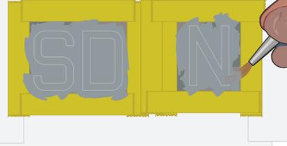
**5** Carefully remove outer paper and tape masking, followed by the mask itself. If care is taken, the masks can be reused several times. Use either a scalpel or pick to do this.
