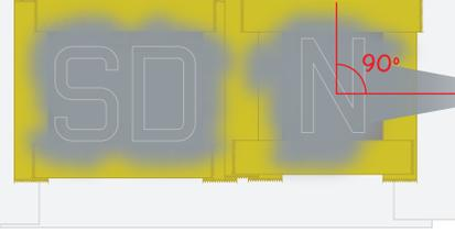
Application option 2: Hand paint appropriate colour (in this case Medium Sea Grey). If applying over a darker colour, it may be beneficial to apply a matt white base coat first. Our masks also include components with slightly irregular edges to give a rougher field-applied effect. In both cases, apply in thin layers to avoid raised surfaces.
